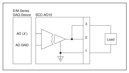
Figure 1. SCC-AO10 Connected to a Nonreferenced Load
